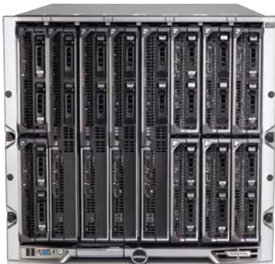
Dell PowerEdge M1000e Chassis
